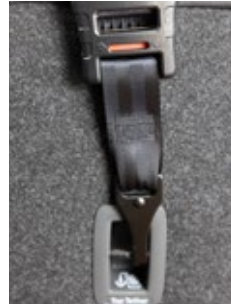
Top tether strap to provide extra restraint and stability. Green indicates top tether is correctly fitted, red indicates incorrect fitting.
