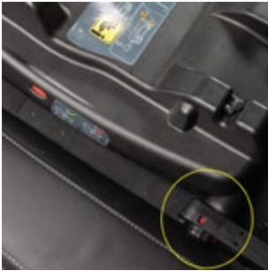
Red indicators to tell you it's not properly connected
