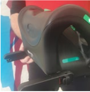
ISOFIX connectors on the child car seat
