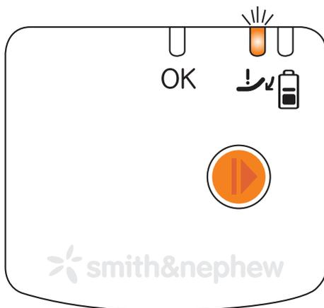
The orange light will flash like this if the pump cannot reach the proper vacuum level.
